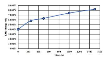
•500 hours constant temperature and humidity load characteristics (Temperature 40°C, humidity 95%)
